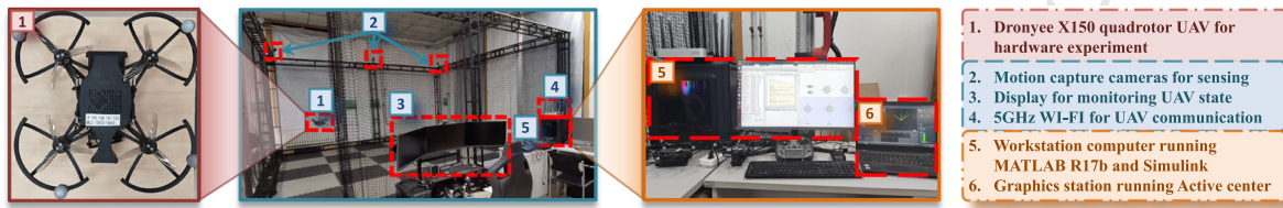
Fig. 3 Hardware equipment used in the UAV tracking control experiment
